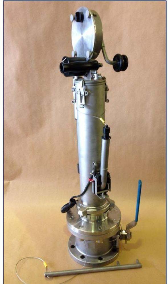
In operation, the winder is mounted directly onto the vessel's vapour lock valves (coupling is provided to suit).
