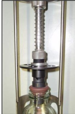
Inlet valve set to minimum opening
