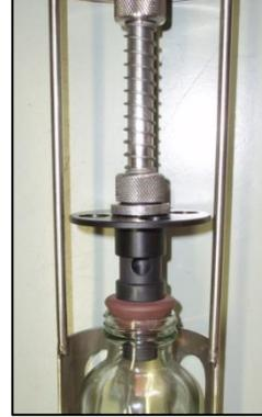
Inlet valve set to maximum opening
