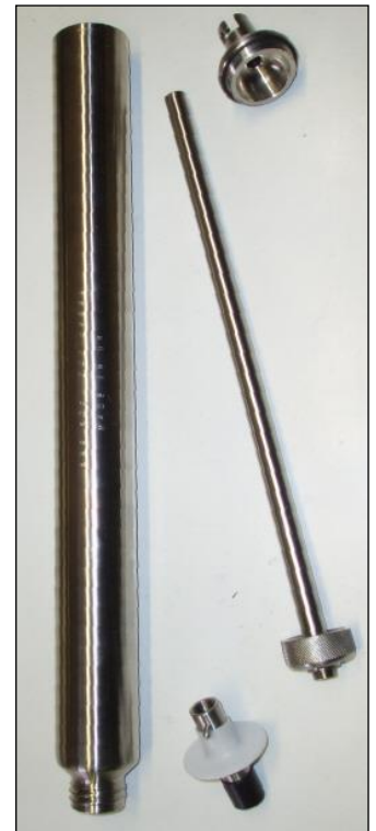
RNS 502 D (Dismantled for cleaning)
