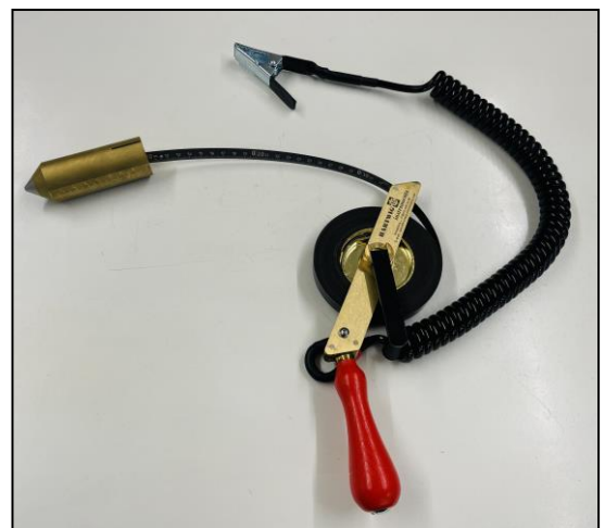
30m tape on frame with 0.7kg weight and earthing strap
