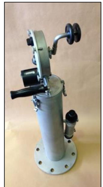
Main tube, showing vacuum pump and support strut
