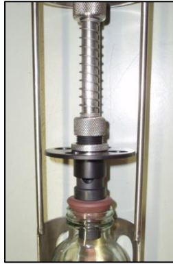
Inlet valve set to minimum opening (for light products)
